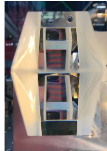
Figure 6.8: Picture (left) taken down the axis of the beamsplitter towards a mirror, as shown in the diagram (right). The interference fringes are visible in this picture, indicating that the two beam paths through the beamsplitter (as shown in diagram on the right) are equal.
